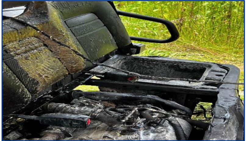
Fire damage underneath the UTV’s seat.
